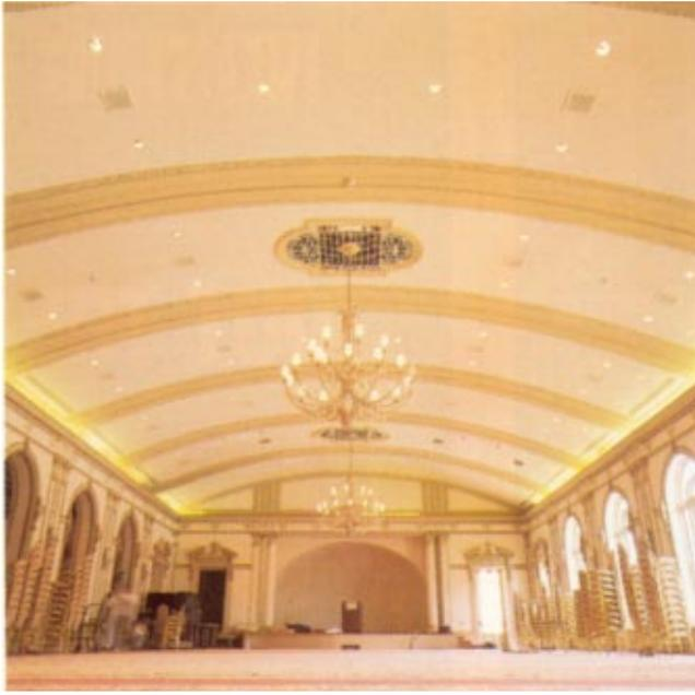
*Veneer plaster systems were used extensively in the recent renovation of the Stouffer Vinoy Hotel, in St. Petersburg, FL. More than 15,000 sq ft of basecoat and lime/gauging plaster were installed over the walls and ceilings of the hotel's restored ballroom.*
